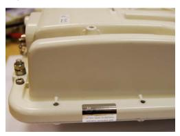
Figure 1-23 Tamper evident label on top edge of ODU
