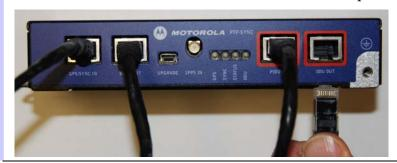
6 Use a grounding cable to connect the ground stud of the PTP-SYNC to the master ground bar of the building.
