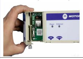
Plug in the cable from the LPU (or PTP-SYNC if installed), ensuring that it snaps home.
