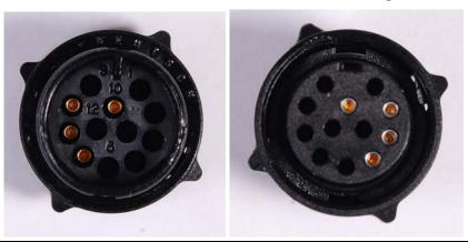
Insert the eight contacts into the connector body in accordance with Table 5-1. It is easiest to insert the pins from the inside out, in the order 12, 11, 9, 5, 4, 3, 2, 1. Push the contacts in so that the shoulder on the contact fits into the hole in the connector shell. When all contacts have been fitted, push them in further to engage with the locking mechanism in the connector shell. This can be done by applying pressure to the contact with a small diameter stiff object, such as tweezers.
