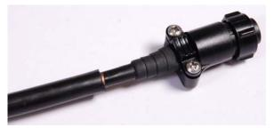
8 Connect the adapter to the GPS, then wrap a layer of self-amalgamating tape, starting 25mm below the bared back outer of the cable and finishing at the GPS housing.
