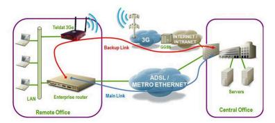
The right figure illustrates the Teldat 3Ge VoIP to GSM Mediagateway capabilities. The enterprise router is featured with a SIP Proxy and the Teldat 3Ge formats the VoIP call into a GSM audio call.
