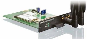
The 4G Europe/Australia Module allows using all current mobile phone technologies with every Viprinet Multichannel VPN Router in Europe and Australia. LTE is the newest mobile phone standard available worldwide — also called 4G. It allows higher bandwidths and higher ranges at the same time and forms the current state of the art regarding mobile phone services. Thus, it provides long-term feasibility.
