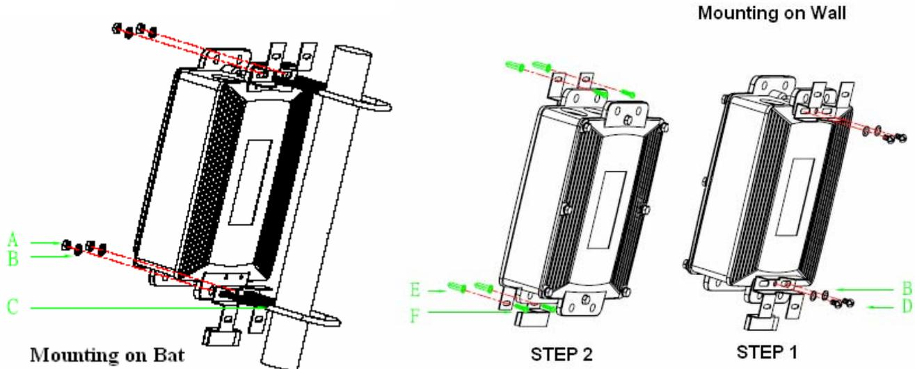
1. Connect desired N-type antennas to the corresponding N-type connectors on the upper panel.
