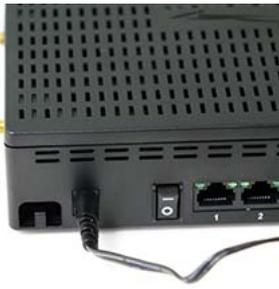
1. Connect the power supply to the router and then plug the other end into an electrical outlet.
