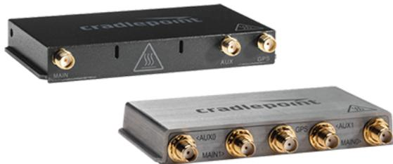
The AER1600 includes a slot for an additional MC400 modem. This enhanced capability allows for redundancy, advanced configuration, failover, and upgradability. The AER1600 supports both the MC400-600M or the MC400-1200M. Refer to the following for more information:
