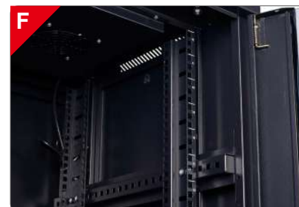
Front and rear sets of vertical rails adjust in quarter inch increments. Adjustment is quick and convenient. Simply unscrew the rails, adjust them to the required depth and re-fasten.
