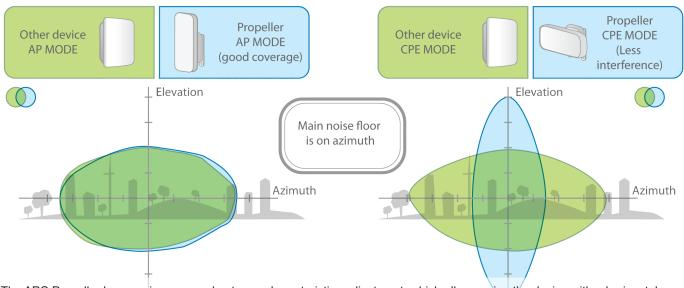
The APC Propeller has a unique manual antenna characteristics adjustment, which allows using the device with a horizontal orientation for client mode. This greatly reduces interference, as the main noise source is on the azimuth. Alignment is easy as only left and right movement of the device is necessary (no need to move it upwards or downwards as the antenna angle on the elevation is wide).
