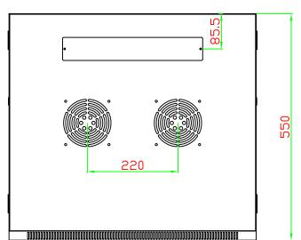
Partcode: CAB15WB550BLK Colour: Black RAL9005 Loading capacity: 40kg
