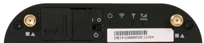
SIM SLOT/ON-OFF / LEDs / SIGNAL STRENGTH COR IBR600
