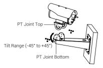
Figure 2-5 Secure the PT Joint
