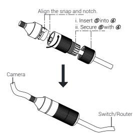
Figure 2-13 Water-proof Accessory Installation
