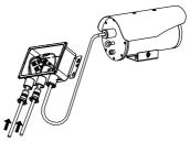
Figure 2-10 Install the Camera onto the Junction Box
