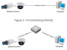
Figure 2-15 Connecting via a Switch or a Router
