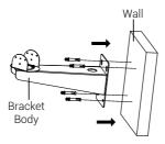
Figure 2-2 Fix the Bracket Body
