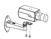
Wiring, adjust the screws to adjust the camera's direction.
