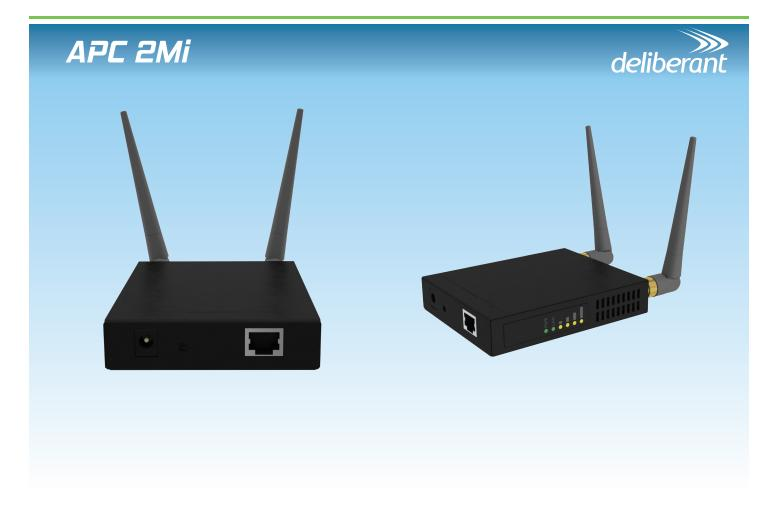
The APC 2Mi is a small, but robust and high performance 2.4 GHz access point designed for indoor applications. This product is equipped with an extreme output power (up to 30 dBm) 802.11n MIMO radio which allows communicating effectively older 802.11b/g equipment together with latest standards wireless devices. The APC 2Mi is coupled with an advanced and featurerich operating system which allows the product to operate as an access point and as a station at the same time, also
