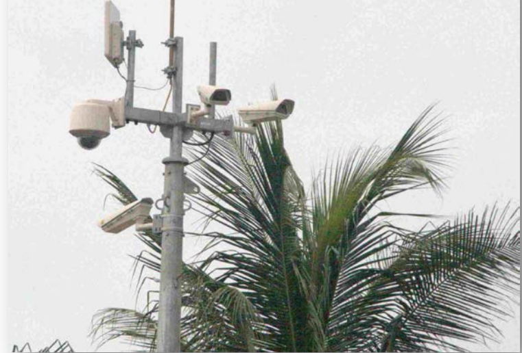
3 Cameras (2 Fixed, 1 PTZ) – 10 Mbps by HSU 520
