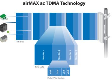
*Up to 100 airMAX ac stations can be connected to an airMAX ac Sector; four airMAX ac stations are shown to illustrate the general concept.*
