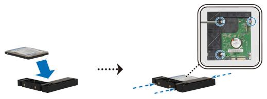
**b** Slide the 2.5" Disk Holder into the hard drive bay, and push it all the way until the drive is firmly connected to the SATA connector. Secure the Disk Holder with the screws provided.
