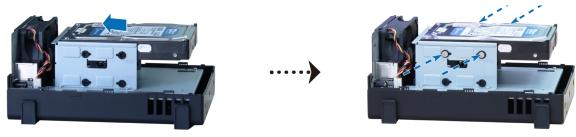
• For 3.5" drives with 2 screw holes on each side (indicated below):
