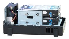
**Note:** If you want to create a RAID volume, we recommended that all installed drives are of the same size to make the best use of drive capacity.
