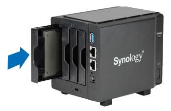
*Important:* Make sure the drive tray is completely inserted. Otherwise, the drive might not function properly.
