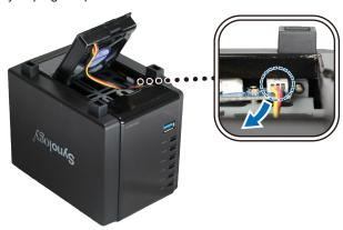
4 Remove the screws from the fan case and slide out the malfunctioning fan.
