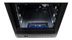
**Note:** When you remove the drive trays, sensitive internal components are exposed. Avoid touching anything other than the memory assembly when removing or adding memory.
