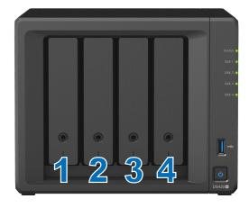
**Note:** If you plan to create a RAID volume, we recommend installing drives of identical size to make the best use of drive capacity.
