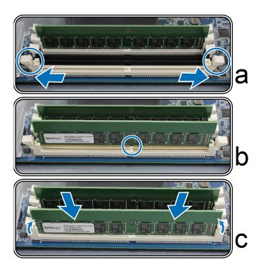
Important: Hold the memory module by its edges. Do not touch the golden connectors.
