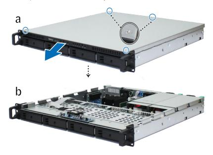
**Note:** When you remove the top cover, you expose sensitive internal components. Avoid touching anything other than the memory assembly when you remove or add memory.
