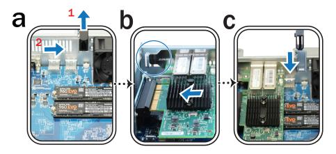
Note: Make sure the connector is fully inserted or the network interface card may not function properly.
