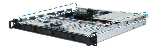
2 Fasten the four removed screws in step 2 of To install a RAM module.
