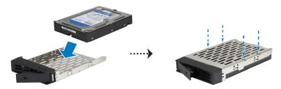
• For 2.5" drives: Place the drive in the drive tray. Turn the tray upside down and tighten the screws into the four spots indicated below to secure the drive.
