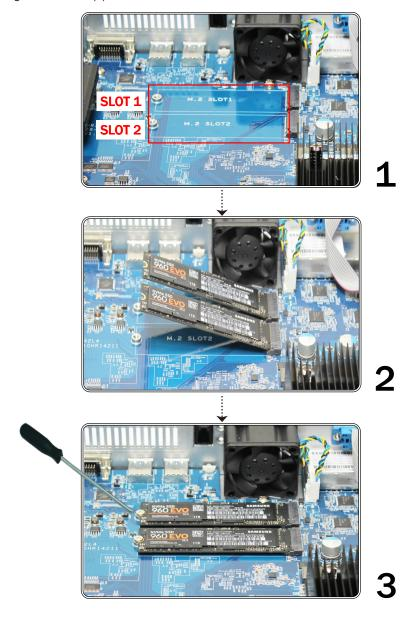
*Important:* Hold the SSD module by its edges and do not touch the golden connectors.
