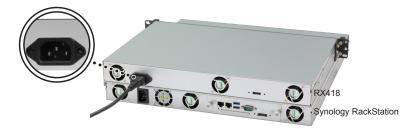
2 Connect one end of the expansion cable to the expansion unit, and the other to the main RackStation unit.
