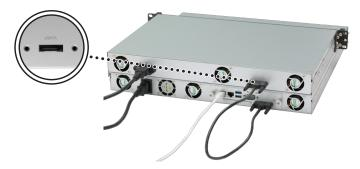
After the connection is complete, the expansion unit will be turned on or off automatically when the connected RackStation powers on or off.
