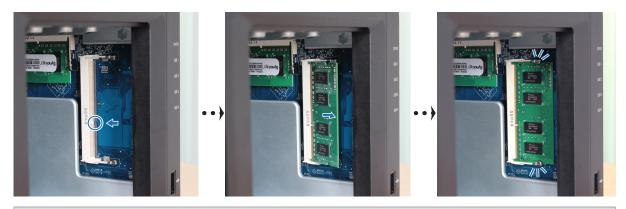
Important: Hold the memory module by its edge, and do not touch the gold contacts.
