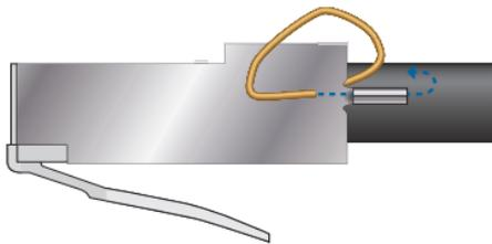
11. Crimp the drain wire hook with a pair of needle-nose pliers to create a secure contact between the drain wire and hook.
