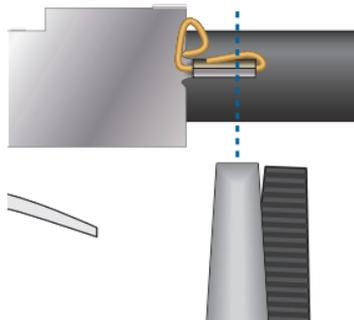
**TC-GND Users** - If you are using TC-GND TOUGH Cable Connectors, then secure the end of the ground wire to a grounding point, such as the tower ground system or a metal mounting bracket.
