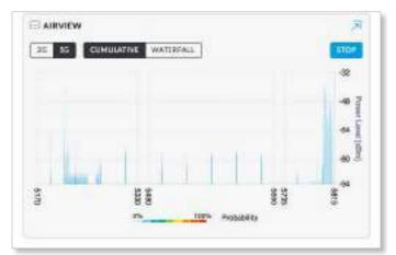
• Waterfall Select Waterfall to track the aggregate energy collected since the start of the airView session for each frequency. The power of the energy (in dBm) is displayed across the frequency span, and a new row is inserted every few seconds.
