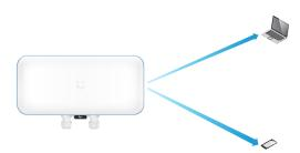
MU-MIMO with 3x3 and 1x1 clients: Each client radio of the UniFi WiFi BaseStation XG communicates with one 3x3 client and one 1x1 client at a time.
