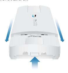
2. Connect an outdoor, shielded Ethernet cable to the *DATA* port.
