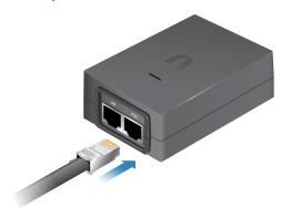
4. Connect an Ethernet cable from your network to the Ethernet port labeled **LAN** on the *airFiber PoE Adapter*.
