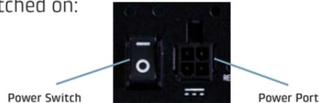
When you set the power switch to the ON ( I ) position, watch for the power LED to illuminate.
