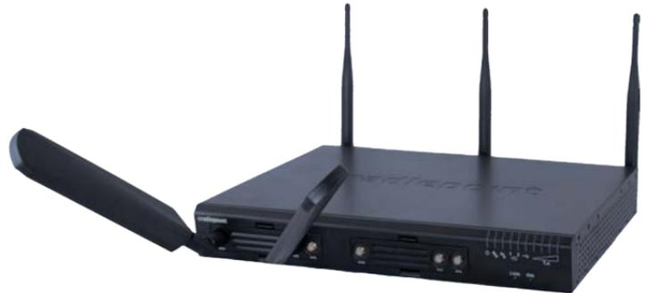
Care should be taken to ensure that the router antennas are not near metal or other RF reflective surfaces. Do not mount router on a wall.
