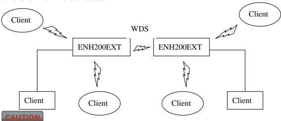
Not every Access Point device has support WDS in Access Point Mode. It is recommended using ENH200EXT if you would like to use this service.
