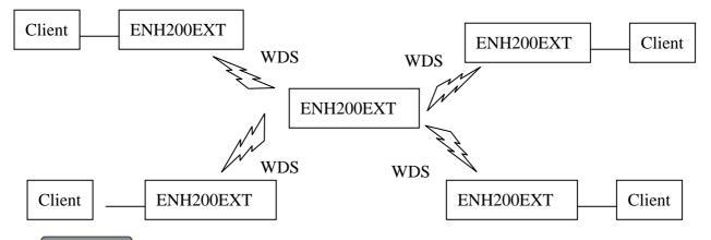
WDS Bridge Mode is unlike Access Point. APs linked by WDS are using the same frequency channel, more APs connected together may lower throughput. Please be aware to avoid loop connection diagram, otherwise enable Spanning Tree Function.
