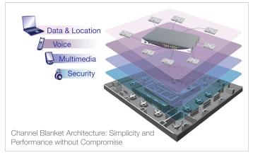
The EXSW-800G takes full advantage of 802.11n, with every port supporting Gigabit Ethernet. The Extricom WLAN system enables a gradual introduction of 802.11n into the enterprise. Using Channel Blankets to separate 802.11n clients from legacy 802.11a/b/g clients provides full performance for all. And only Extricom allows co-existence of both 802.11n and legacy 802.11 b/g devices in the 2.4 GHz band without throughput degradation for either type of client.
