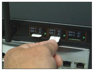
Note: Order of insertion for SIM cards must be slots SIM 1, SIM 3, SIM 5
