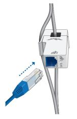
Connect the other end of the CAT5/6 cable from the mFi Current Sensor to an mFi RJ45 port on the mFi mPort.
