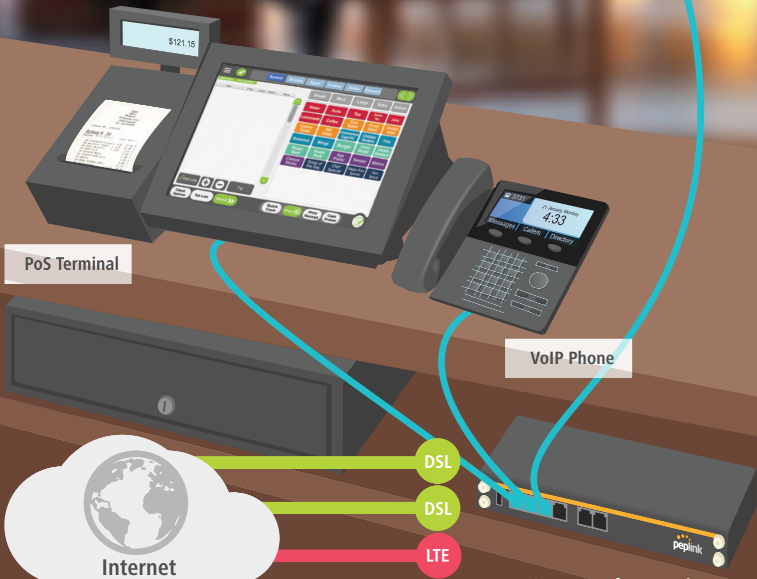
Failover Between 2x DSL and 1x LTE Links
