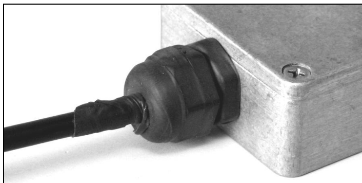
Figure 35: Weatherproofing LP Ethernet Cable Entry - Pt-2
