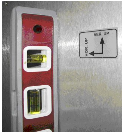
Figure 38: Antenna Alignment - Levelling Antenna Elevation Plane
