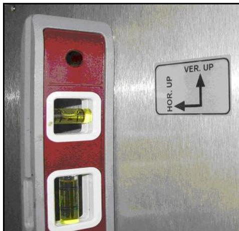
**Figure 40: Procedures - Antenna Alignment - Zero the Antenna Elevation Plane**
