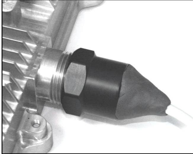
**Figure 27: Procedures - Ethernet Port - Weatherproofing Pt-1**
