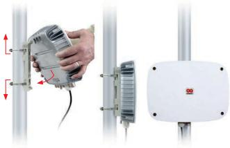
**6** Attach bracket to the mast using hose clamps. Clamps shall be as much to the outer edge of bracket, as possible.
