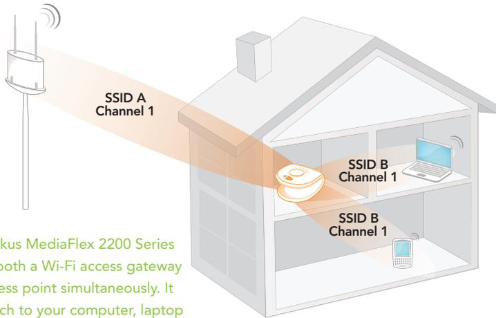
The Ruckus MediaFlex 2200 Series acts as both a Wi-Fi access gateway and access point simultaneously. It can attach to your computer, laptop or networking hub using an Ethernet cable or via a wireless 802.11g link.
