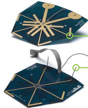
A state-of-the-art smart antenna array controlled by an expert software system integrates six high-gain horizontally-polarized antenna elements and two vertically-polarized antenna elements. This provides a 7 dBi gain thereby delivering unprecedented range extension and Wi-Fi signal reliability. The best antenna elements are used at any given moment for any given packet and any given client based on changing environmental conditions.
