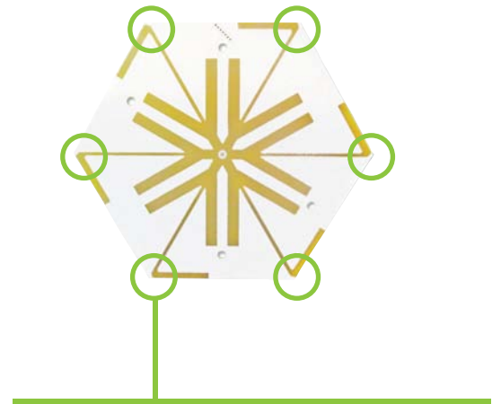
Six high-gain directional antenna elements controlled by an expert software system that determines the best antenna pair for any packet at any given time
