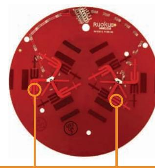
The high-gain directional antenna system specifically designed for spatial multiplexing, a technique used by 802.11n, provides multiple antenna elements that are controlled by an expert software system. This system determines the best antenna pair for any packet at any given time
