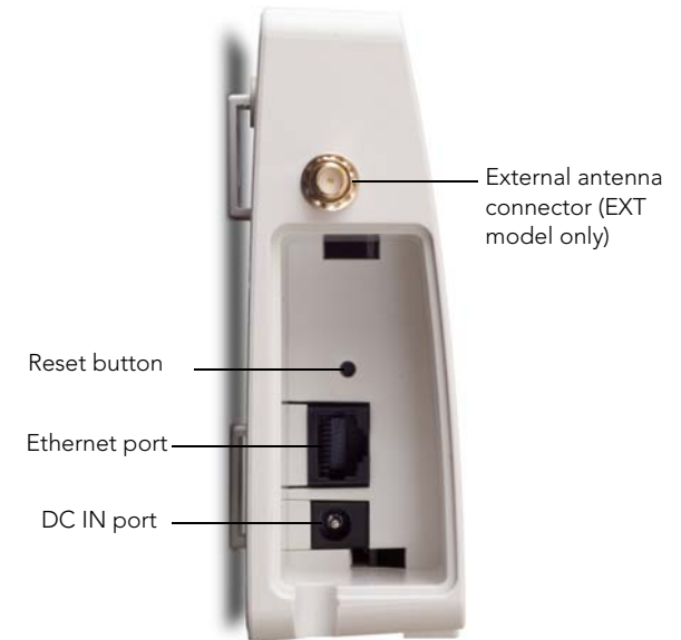
Figure 1. Side panel of Indoor/EXT Smart Wi-Fi Gateway
