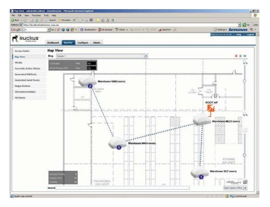
First-time users plug their computers into the LAN and specify a URL that directs them to a captive web portal for a one-time authentication. After successful authentication, the ZoneDirector automatically configures the client system with the designated SSID and a dynamically-generated encryption key. The key is bound to the client, and can be removed upon expiration when the user or the user's device is no longer trusted.
