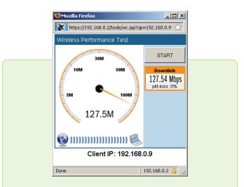
SpeedFlex<sup>™</sup> is a unique wireless performance test tool integrated within the ZoneFlex<sup>™</sup> family of centralized controllers that measures the Wi-Fi throughput of associated wireless LAN clients.
