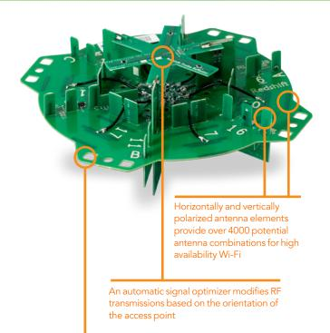
A patented smart antenna array integrates high-gain, directional antenna elements deliver up to 7dBi in signal gain and up to -15dB of interference avoidance for unprecedented range extension, signal reliability and higher data rates.
