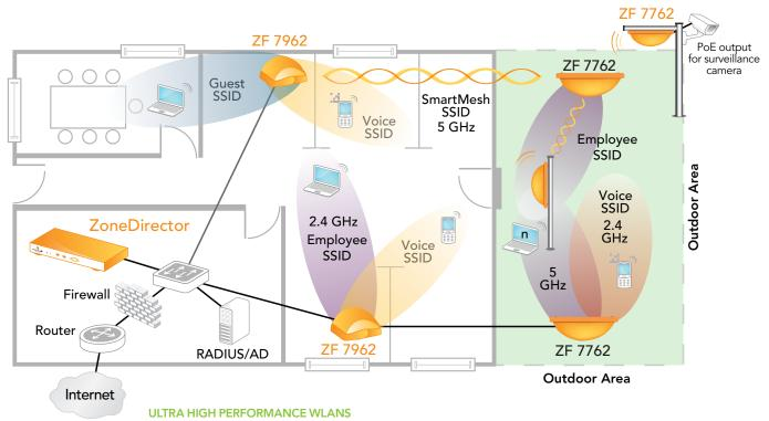
Through the use of an integrated smart antenna array specifically designed for 802.11n networking, the Ruckus ZoneFlex 7962 provides the industry's highest performing enterprise WLAN solution. WLANs can be easily extended where Ethernet is unavailable through the use of Smart Mesh Networking.
