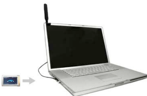
Laptop equipped with Ubiquiti SRC + external antenna
