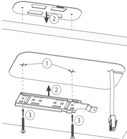
A Special bracket is included in the package to mount on the drop ceiling. As it consists of two parts, to be attached on both sides of the ceiling tile.
