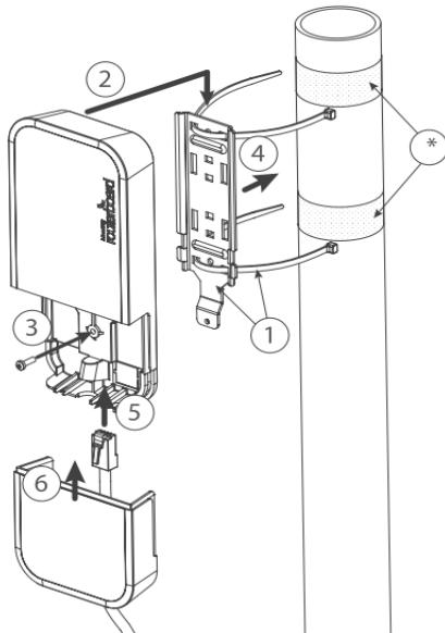
\* It's recommended to use electrical tape to increase friction between materials.
